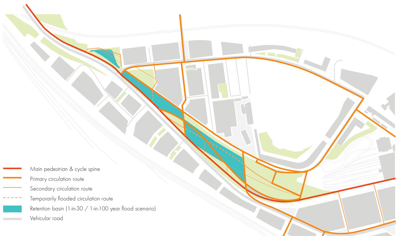
Fig.61 Retention basin levels are to be designed so as to ensure primary pedestrian circulation routes are not compromised in a flood event
